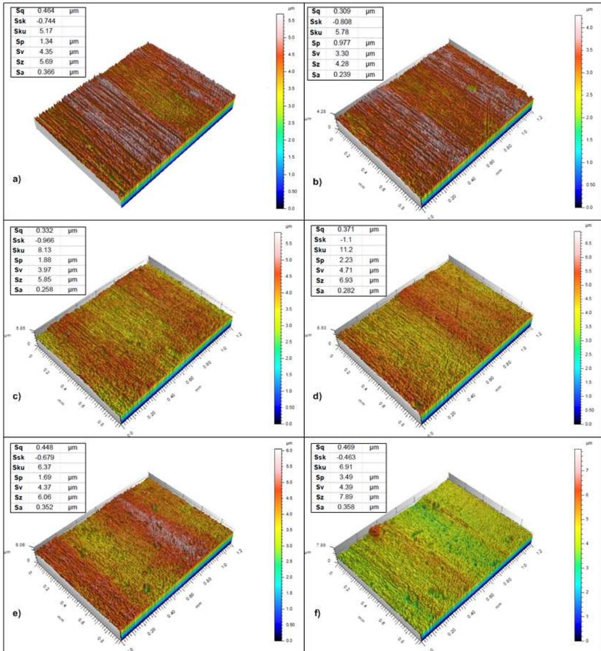
Fig. 4. 3D isometric views and statistic characteristics (ISO 25178) of AISI4130 cylinders surfaces for different 1<sup>st</sup> (a), 2<sup>nd</sup> (b), 3<sup>rd</sup> (c), 4<sup>th</sup> (d), 5<sup>th</sup> (e) and 6<sup>th</sup> (f) level of burnishing conditions.
