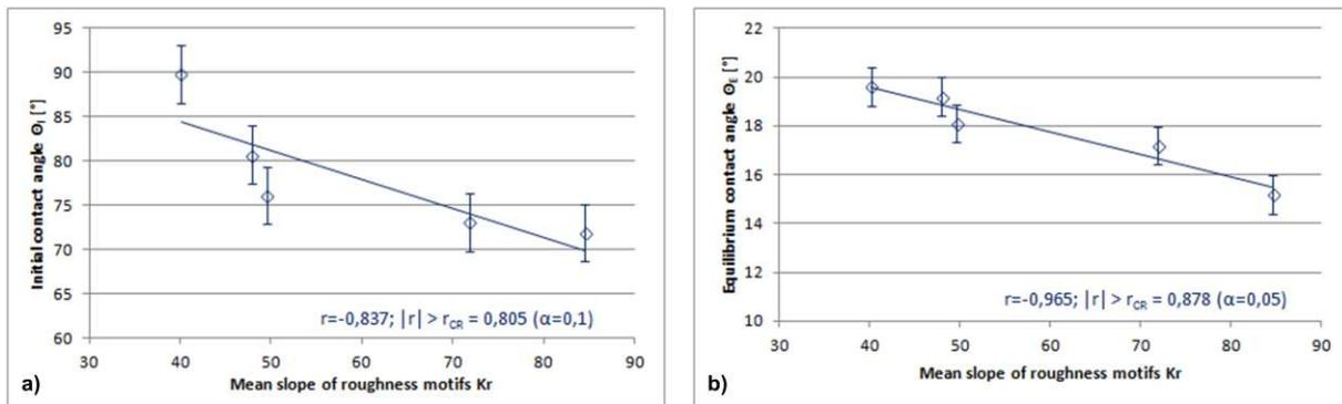
Fig. 6. Initial contact angles  $\Theta_I$  and "balance" contact angles  $\Theta_E$  versus mean slope of roughness motifs  $K_r$  ( $r$ -Pearson correlation coefficient,  $r_{CR}$ - critical value for Pearson correlation,  $\alpha$ -statistical significance).
