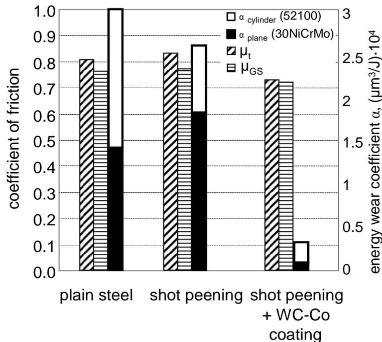
Figure 4: Evolution of the coefficient of friction:  $\mu_t$  - at the transition between partial slip and gross slip,  $\mu_{GS}$  - in full sliding gross slip conditions and quantification of the wear volume based on a dissipated energy approach (cylinder/plane configuration).
