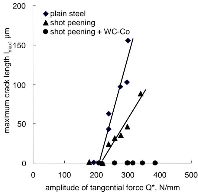
Figure 6: Fretting wear cracking nucleation and propagation evolution of studied tribo-systems under partial slip conditions (cylinder/plane configuration).
